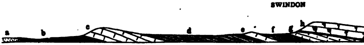
FIG. 1566. — Diagrammatic section across England from Gloucester on the west to Swindon on the east, showing the succession of Mesozoic formations. a , Triassic; b-g , Jurassic ( b , Lias; c , Lower Oölites; d , Oxford Clay; e , Corallian; f , Kimmeridge Clay; g , Portland and Purbeck beds); h , Cretaceous (Chalk). (From Lake and Rastall, Text-book of Geology .)
